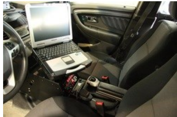
Toughbook 31 fully rugged laptop, PMT TrimLine CF-31 vehicle dock, mousetrap motion mount and PMT SightLine console in Ford Police Interceptor sedan
