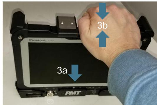
\*Avoid holding the tablet in the top corners while docking to prevent potential pinch point with corner ears.
