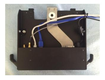
Connect all cables securely to dock connections, and use tie straps to secure cables to the built-in slots on the mounting/interface plate.
