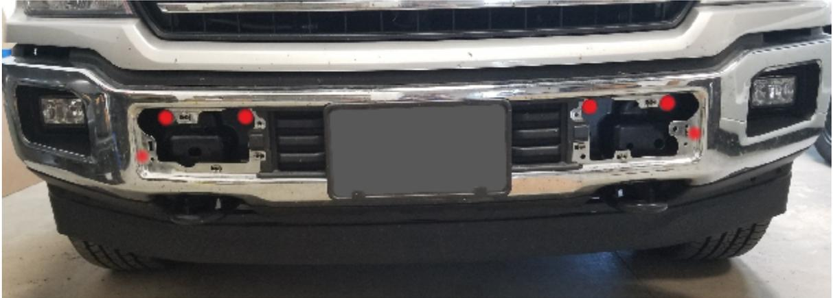
2. Remove tow hooks on both sides from vehicle (if necessary) by removing all (4) bolts with a 5/8"socket. Save all bolts and both nut plates for later use. (Extra bolts and nut plates have been provided in hardware bag for vehicles without tow hooks).
