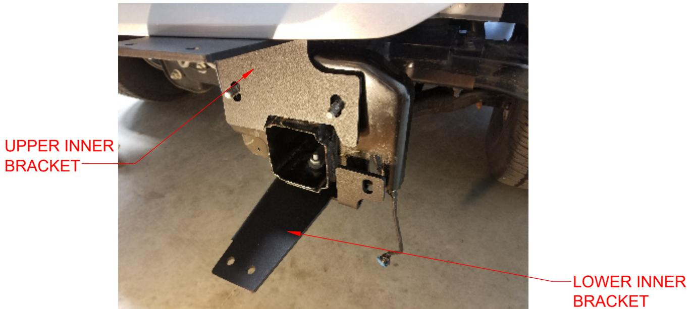
4. Reinstall the bumper, making sure lower bracket fits through tow hook hole in bumper. Reinstall front (4) factory nuts, making sure bumper is fully lifted into place. Loosely reinstall back (2) factory nuts. Reconnect all lights and plugs.
