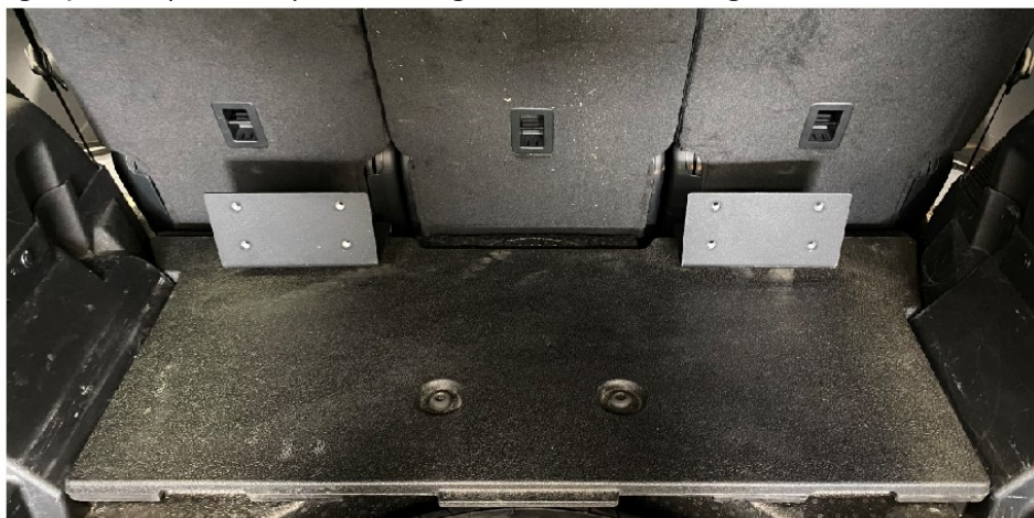
Fig.9 IMAGE FROM REAR END CARGO PANEL INSTALLED
