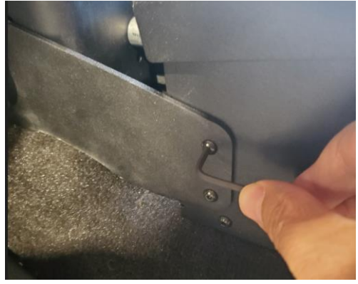
b) Install the side supports using socket set suitable for #10-24 screw.
