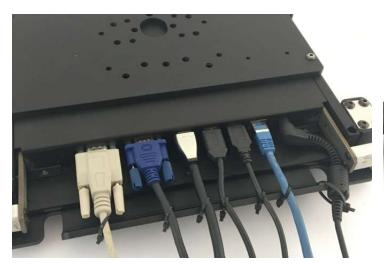
Connect all cables securely to dock connections, and use tie straps to secure cables to the cable tie rail. Ensure to leave enough slack in wires exiting dock so that any positioning adjustments will not strain the cables or connections.
