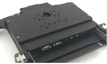
The standard mounting bracket that comes with the vehicle dock features an industry standard VESA 75mm x 75mm bolt pattern. This allows easy mounting to many preexisting mounts as well as dedicated mounts from PMT. Use the supplied #¼-20 hardware for attaching it to the mount.
