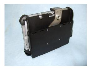
The standard mounting/interface plate that comes with the PMT G1 TrimLine vehicle dock features an industry standard VESA 75mm x 75mm bolt pattern. This allows easy mounting to many pre-existing mounts as well as dedicated mounts from PMT. The screws needed for this are M4 x 12mm.
