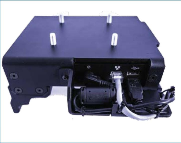
Connect all cables securely to dock connections. Use cable ties to secure cables to the built-in cable tie slots.
