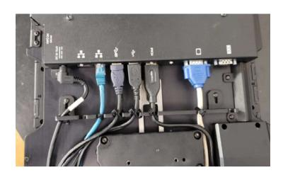
Connect all cables securely to dock ports, and use tie straps to secure cables to the "Cable Management Bar" as shown.
