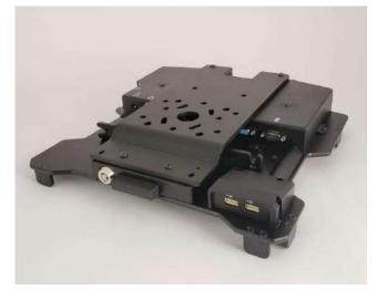
The standard mounting bracket that comes with the vehicle dock features an industry standard VESA 75mm x 75mm bolt pattern. This allows easy mounting to many preexisting mounts as well as dedicated mounts from PMT. Use the supplied #¼-20 hardware for attaching it to the mount.
