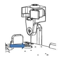
**NOTE:** The Screen Lock arm might get loose after repetitive use (10,000 cycles). If the arm gets loose, tighten the ½-20 screw, as shown to the left, to desired torque using an allen key
