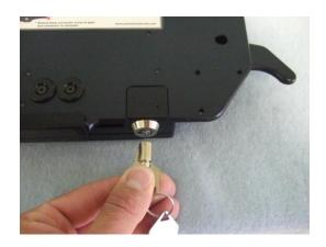
Step 3: Rotate the key 90 degrees clockwise until it stops, and remove the key
