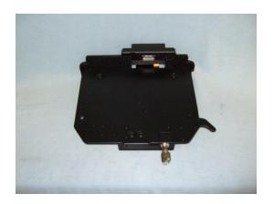
It is now possible to remove the key from the dock while leaving the dock in it's "open" configuration. This protects the docking connector from possible damage, and allows for easy re-docking
