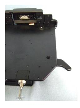
Step 3: The docking lever will spring forward, and the docking connector will retract. Do not proceed with docking the computer until this step is complete
