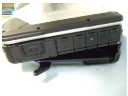
Step 4: Insert laptop front first into the front clamp of the docking station
