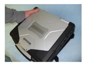
Step 2: Remove the computer by lifting up from the rear of the laptop, and sliding it out of the dock
