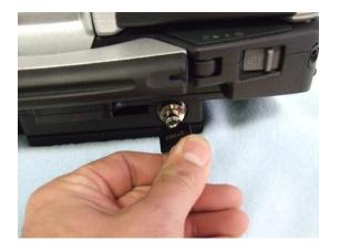
Step 7: While holding the docking lever back, turn the key 90 degrees clockwise and remove the key
