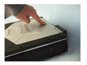
Step 5: Ensure rear of the computer is completely seated by pressing down on the computer
