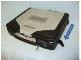
Step 1: Insert key and rotate 90 degrees counter clockwise. The docking lever will spring forward, and the docking connector will disengage
