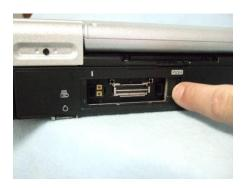
Step 1: Ensure rear connector cover is open on the back of the CF-31 computer
