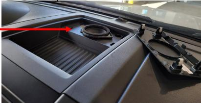
Step 2: Remove two OEM screws by using the 7mm wrench beside the speaker
