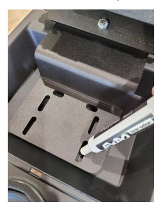
**Step 5**: Drill the marked holes by using  $\Phi 1/4$ " drill
