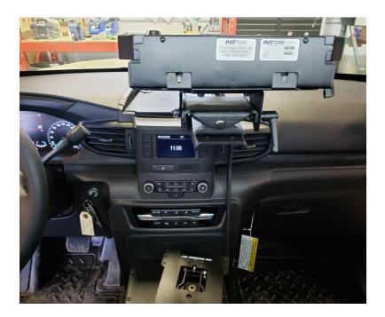
**Step 7:** Pull the latch again to position the tablet dock parallel to vehicle dash screen.
