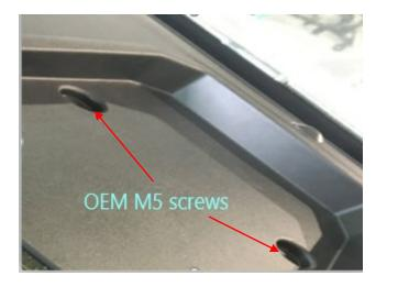
**Step 4:** Install the tablet dock, using the hardware that comes with tablet dock, to the swivel mount plate of tablet mount, as shown in picture. Use #1/4-20 wrench –with related socket set.
