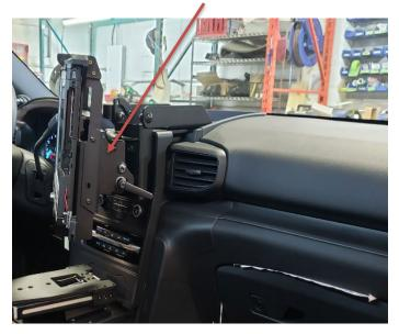
**Step 10:** Ensure to always use the handle to keep the tablet dock to fix in a position tight / firm, which should help in reducing the wiggle while the vehicle is in motion.
