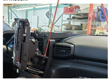
**Step 11:** Attach the dash mount leg on top of console top plate, using 3X #1/4-20 ½" HX SOC BN HD SCREWS and #1/4-20 washers as shown in picture below.
