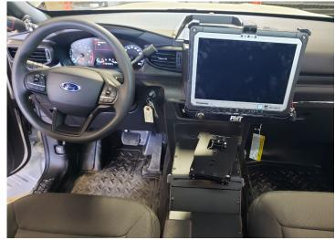
Step 8: The swivel plate shown in picture below will enable the tablet dock to be turned from driver side to passenger side
