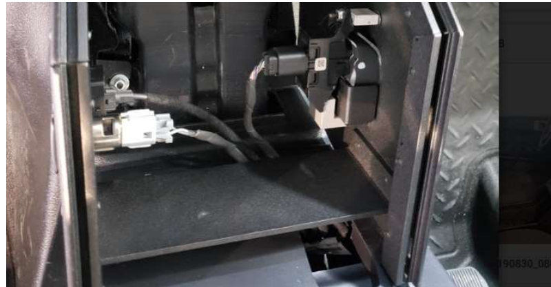
B. Connect back all three cables (E-Brake, USB, and 12V Socket)
