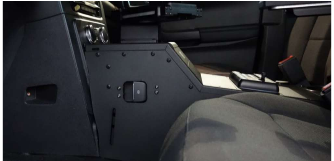
C. Push the console completely in, and make it aligned with the dash.
