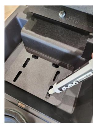
Step 3: Drill the marked holes by using  $\Phi 1/4$  drill
