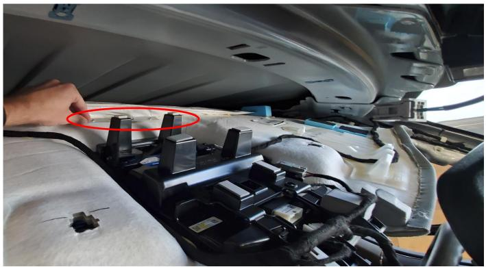
Option2: Gently pry and take off the OEM headliner, and place the headliner back plate in the desirable place.
