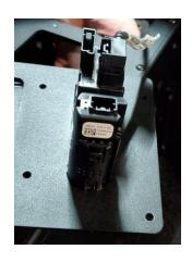
**Step 2.3** Install the rear power port modules to the USB plugs plate.
