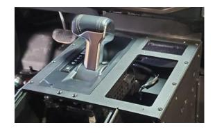
**Step 4**Attach all the wire harness connectors to the ports and vehicle. Test the connections after starting the vehicle.
