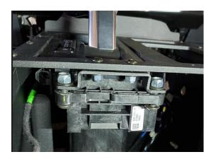
**Step 3.2**Loosely attach the shifter to the front mounting bracket using 5/16-18 X1-1/4 bolts, washers and Nyloc nuts.
