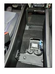
**Step 3.1**Loosely attach the shifter to the rear mounting bracket using 5/16-18 X1-1/4 bolts, washers and Nyloc nuts. Then attach the top plate to the console
