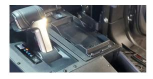
**Step 4.2** Attach the top side trims to the console using #10-32 – 3/8 Phillips PAN Head screws.
