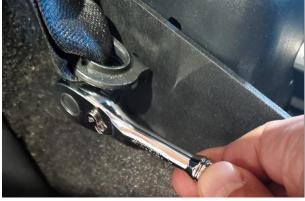
Step 3.1 Install the side supports using socket set suitable for #10-24 screw.
