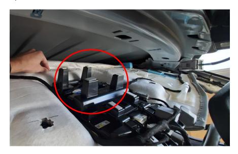
**Option B:** Gently pry and take off the OEM headliner and place the headliner back plate in the desirable place.
