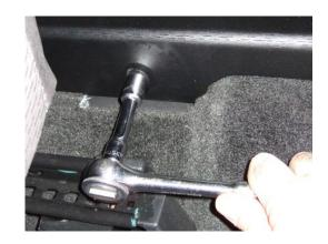
You can now go inside the console and tighten all bolts including the bolts attaching the cross brackets to the console itself.
