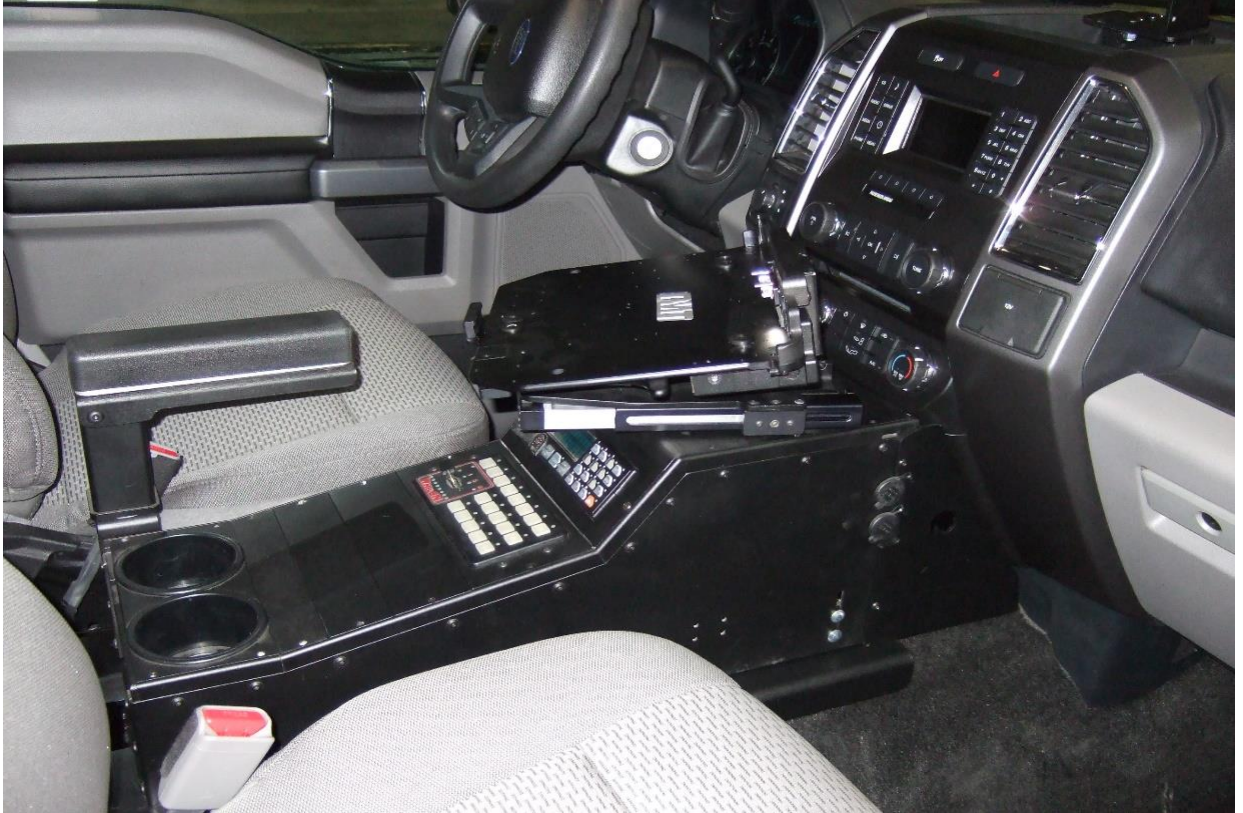
Standard 2015 F-150 console with break-away armrest, trim panels, and Mousetrap Motion Mount
