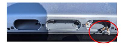
**Step 3**Insert the sandwich plate be rotating and sliding the plate into the center cutout.
