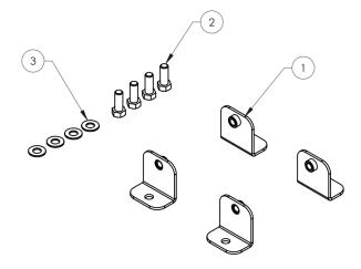
The universal console bracket kit can be used with either the 29" or 23" flanged base plate.
