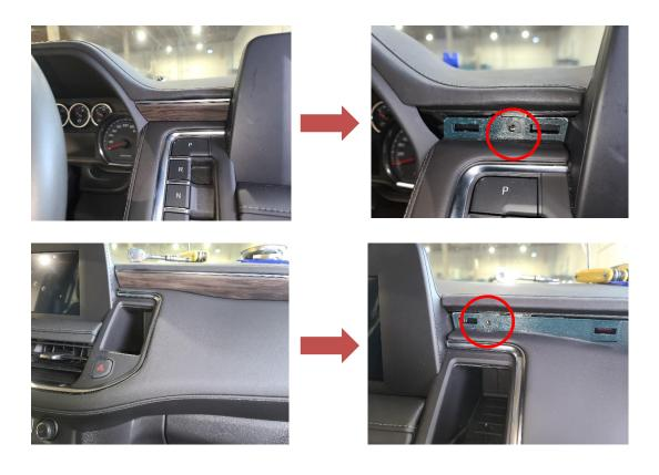
**Step 2**Remove the OEM Hex head bolts on both sides
