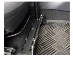
**Step 3**After Universal Base is installed, adjust front support foot as needed
