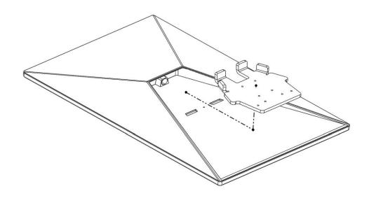
**Step 2**Attach the base plate to the Starlink with the #8-32 hardware.
