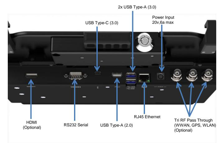
\*RF Antenna connections are optional based on docking station model. Connectors are TNC
