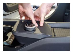
**Step 3** Disconnect the cables and remove the OEM shifter and parking brake
