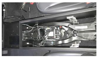
**Step 20** Install the 2 OEM bolts shown to attach the PMT console to the dash
