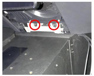
**Step 21** Tighten the 4 front console bracket bolts
