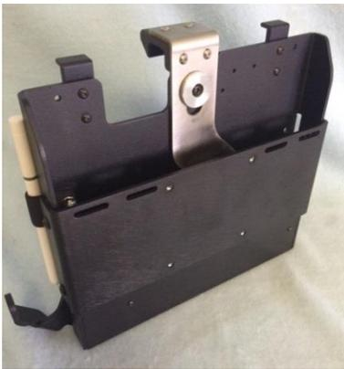
The standard mounting/interface plate that comes with the PMT G1 TrimLine vehicle dock features an industry standard VESA 75mm x 75mm bolt pattern. This allows easy mounting to many pre-existing mounts as well as dedicated mounts from PMT. The screws needed for this are M4 x 12mm.
