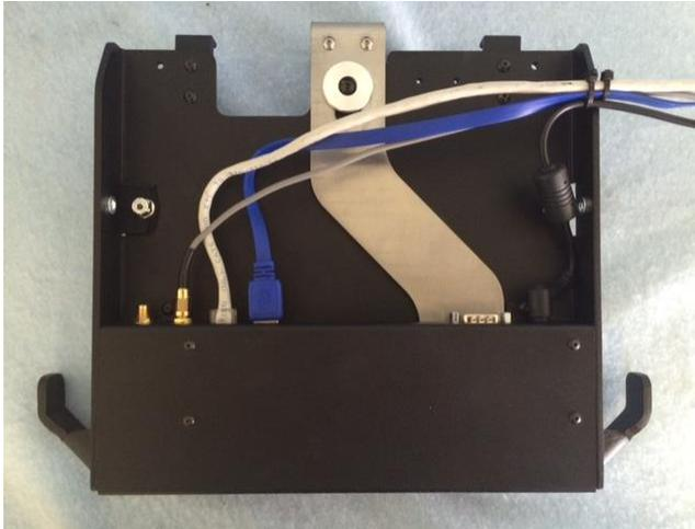
Connect all cables securely to dock connections, and use tie straps to secure cables to the built-in slots on the mounting/interface plate.
