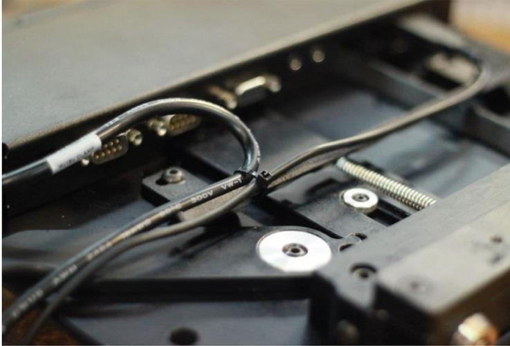
Connect all cables securely to dock connections, and use tie straps to secure cables to the cable tie rail. Ensure to leave enough slack in wires exiting dock so that any positioning adjustments will not strain the cables or connections. Use tie straps to secure opposite cable ends to another location in the vehicle.
